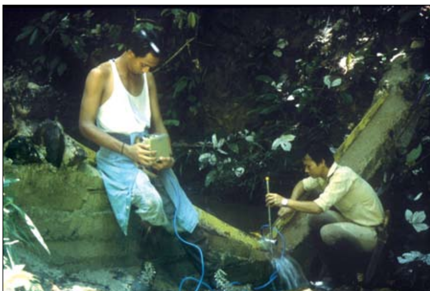
Stream-gauging structure within the buffer zone of the selectively logged Baru experimental watershed, East Malaysia
